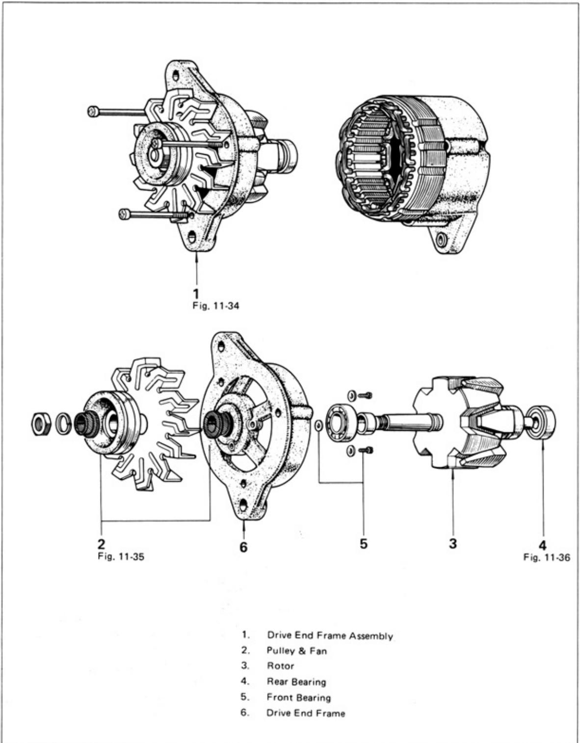
Disassemble the parts in the numerical order shown in the figure.
