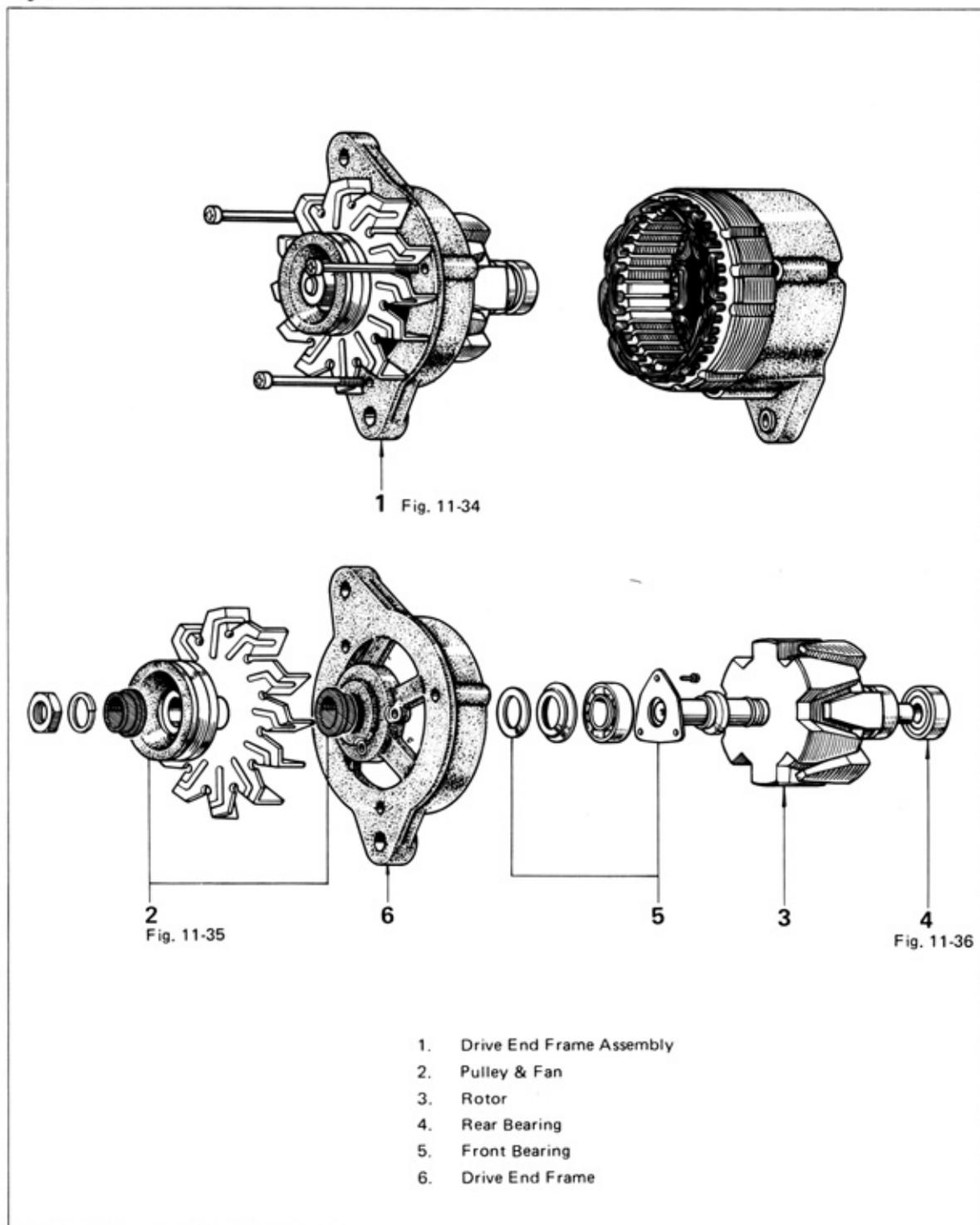
Disassemble the parts in the numerical order shown in the figure.
