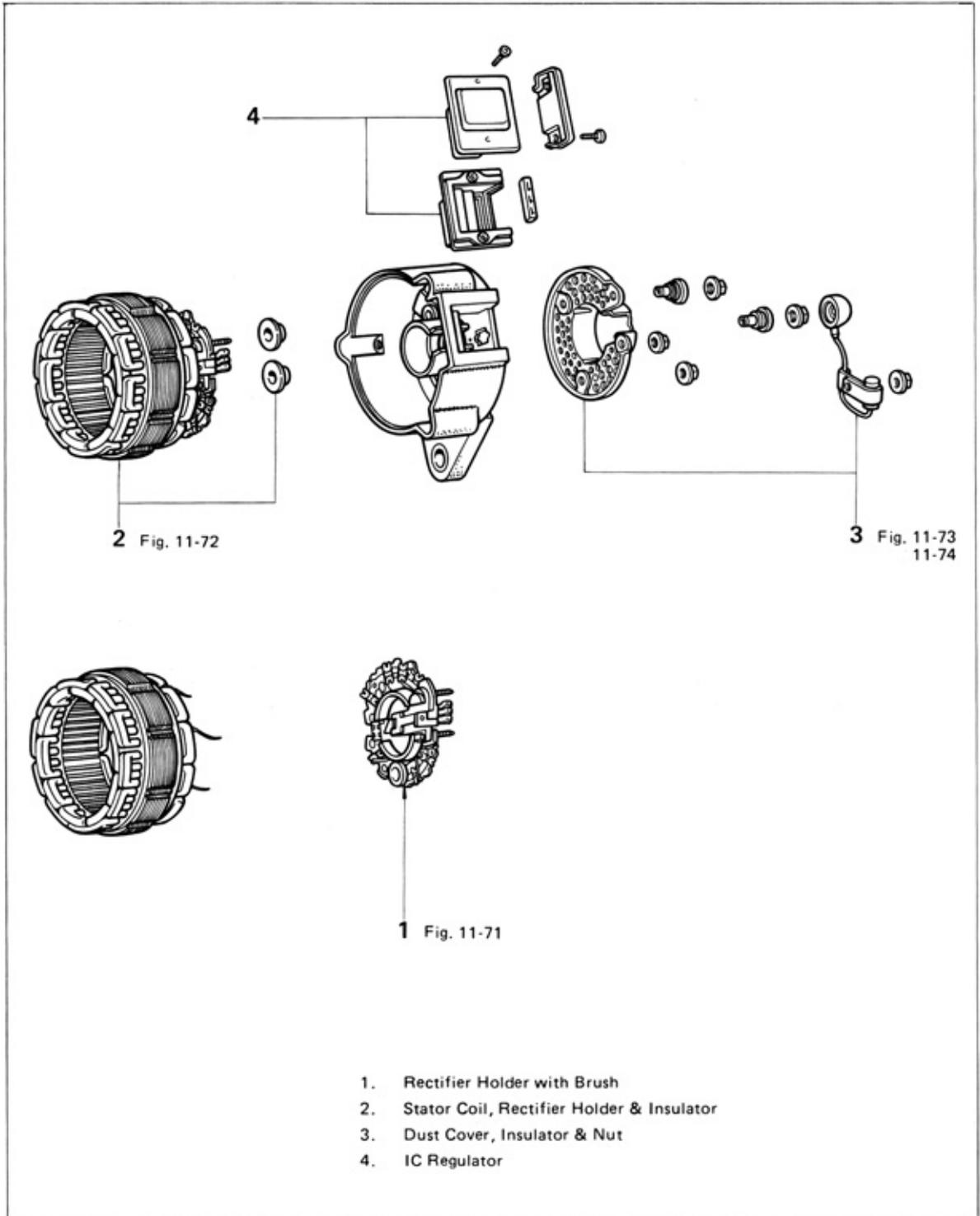
Assemble the parts in the numerical order shown in the figure.
